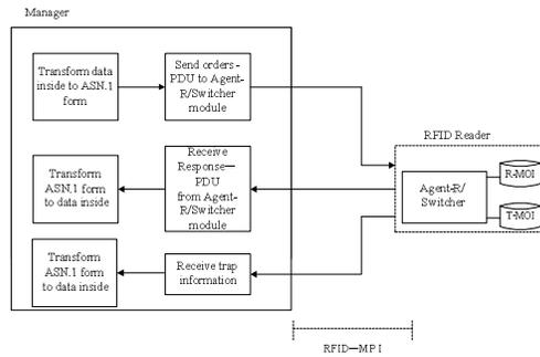
Fig.7 Manager module working principle
