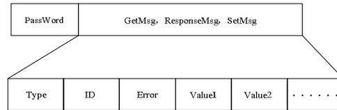
Fig .6 Message transportation form for RFID-MP PDU
