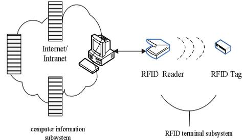
Fig.1 Typical RFID system
