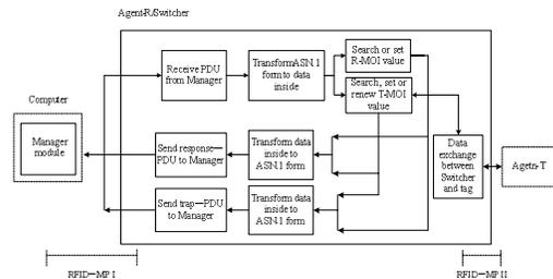
Fig.8 Agent-R/Switcher module working principle
