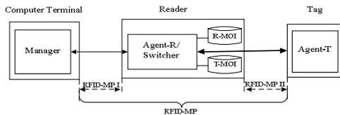
Fig.5 Structure of RFID terminal subsystem management
