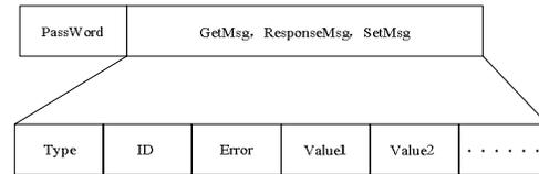
Fig .6 Message transportation form for RFID-MP PDU
