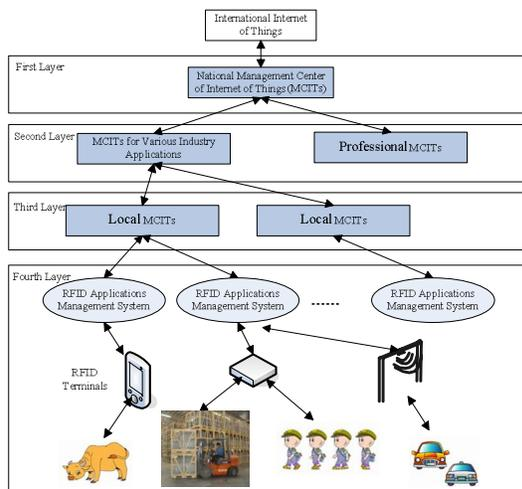
Fig.3 Layered structure for Internet of Things
