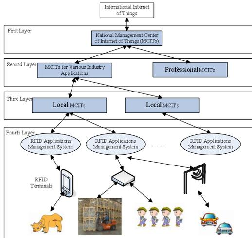
Fig.3 Layered structure for Internet of Things
